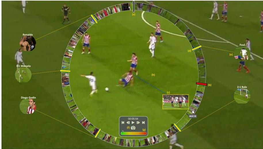
**Fig. 1.** Screenshot of the user interface. (a) start position, (b) playback progress indicator, (c) preview image, (d) bookmark, (e) bookmark preview image, (f) button for setting a bookmark, (g) speed adaptation pad, (h) minimum center distance for navigation (25% of the radius)
